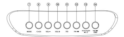
8 CH/ $\bigcirc$ : Button for switching between stations or frequency (in Radio mode);
